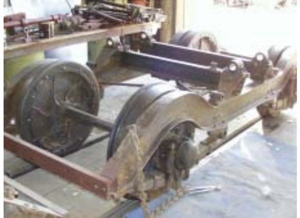
The trucks took many months of hard work to remove all the rust, corrosion and dirt, which were firmly caked to every nook and cranny. The brake levers and linkages were removed and stripped to bare metal to enable them to move freely so the brake shoes can be pressed against the wheels. The trucks are now completely restored, in working order, and re-installed under the car, as is almost all of the brake linkage system. At present we are re-installing the air system that operates the brakes.
